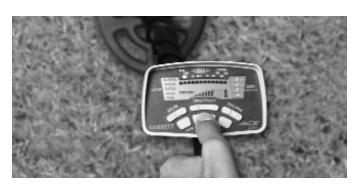
distance between the coil and the ground remains constant throughout the entire pinpointing process; in this case, that distance is zero inches. If the ground's terrain does not allow for this type of "coil scrubbing" then do your best to maintain constant separation between the coil and the ground.
